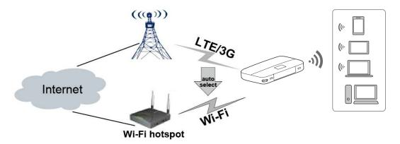
Figure 3-6 LTE/3G/Wi-Fi auto offload
